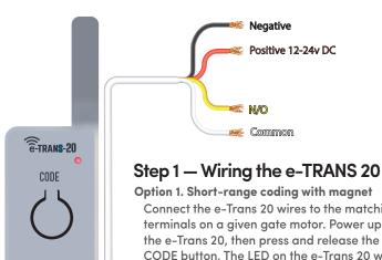
Connect the e-Trans 20 wires to the matching terminals on a given gate motor. Power up the e-Trans 20, then press and release the CODE button. The LED on the e-Trans 20 will light up, now place the magnet on the CODE recess on the e-Loop, the yellow LED on the e-loop will flash, and the LED on the e-Trans 20 will flash 4 times. The systems are now paired, and you can remove the magnet.
