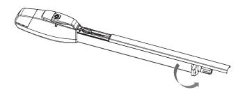
4. Adjust two Knobs to set the open and close position
