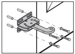
Remove the wire cover and fix the rear bracket with the pin. Release the gate opener and place the pin into the fitting position no.1 and no. 2
