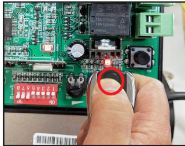
While the light is on, press the first button on the remote control twice.
