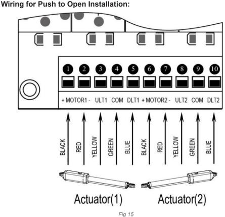
Please Note: To operate the gate as push to open the wires inside the control box for each motor need to be changed to match this diagram (right)
