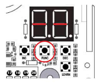
To enter programming mode and change any program settings press and hold the FUNC (function button for 4 seconds. The digital display will flash P1 (Program 1) Meaning you can adjust Program 1 settings.
