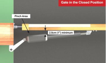
Please Note: Each swing arm contains an internal thread that may separate if overextended. If overextended a "Click" may be heard, to re-connect push and screw the arm Clockwise until the arm begins to retract by hand.
