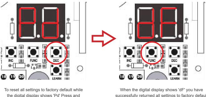
the digital display shows 'Pd' Press and hold the DEC button. When the digital display shows 'dF' you have successfully returned all settings to factory default settings. Press the FUNC button until the "-- --" symbol is displayed to return to operating mode.
