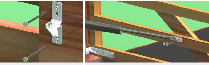
Mark the fance posts through the middle of the bracket slots and drill ø10.5mm holes.
