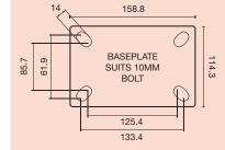
Baseplate dimensions & drilling patterns for Shock-Absorbing castors
