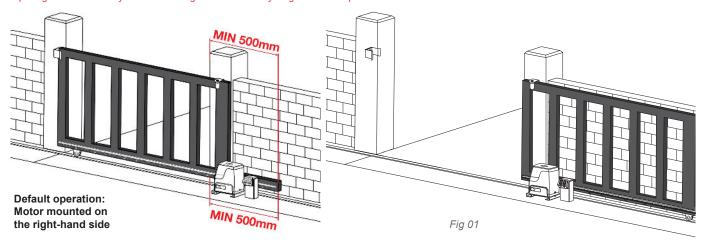
**Before Installing:** Test the motor by plugging it into a power source and pressing the remote. You will see the motor cog turn. When it stops (after approx 1 minute), press the remote again to see it turn in the opposite direction. This will give you an understanding of the way in which the motor will move the gate.
