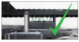
Gear rack correctly aligned at 90° to the motor cog
