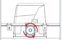
The motor cog will turn counter-clockwise, moving the gate frame.
