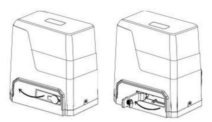
To put the gate motor into manual mode, insert the key and open the manual release bar as shown
