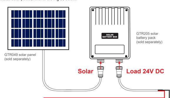
Connect the prestripped black and red wires to the BAT terminal of the GTR207 circuit board, and then connect to your GTR205 solar battery pack using the 2-pin plug supplied.
