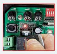
While the light is on, press the first button on the remote control twice.
