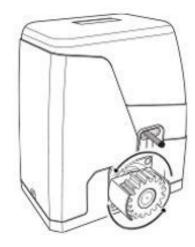
In manual mode, the gear can turn freely and the gate can be operated by hand
