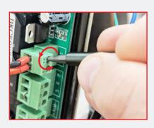
Using a screwdriver, loosen the screw on the side of the terminal.
